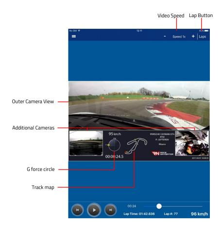
Recorded videos consist of camera views (up to 4 cameras in RN ONE and RN PRO devices) combined with additional data overlay.
